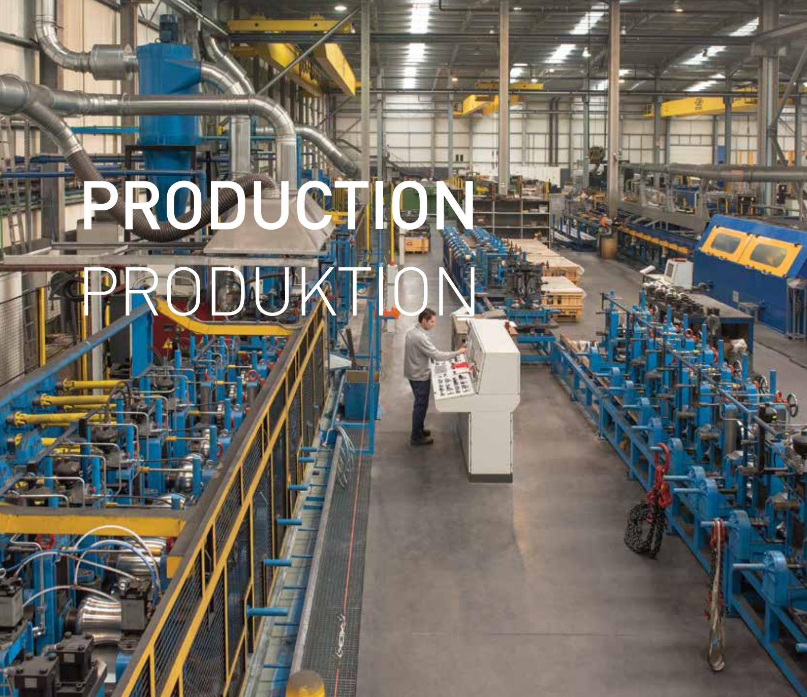
Our tubes are manufactured using high-frequency electrowelding, with no subsequent heat treatment. The entire production process was designed and developed according to the best available technologies, considering environmental and workplace health and safety standards.
